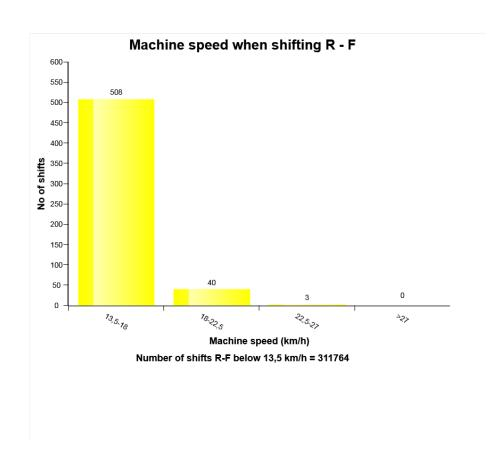
The graph shows the machine speed at direction shift, reverse to forward (R-F)
