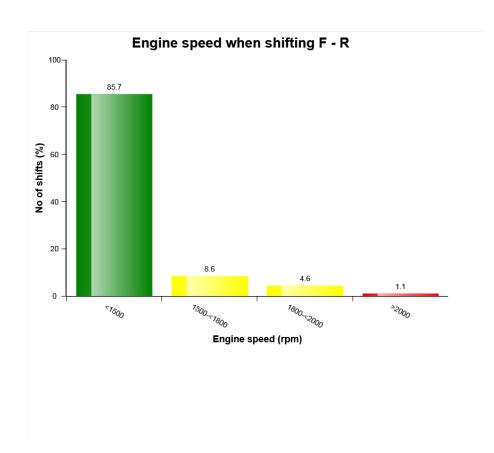
The graph shows the machine speed at direction shift, forward to reverse (F-R).
