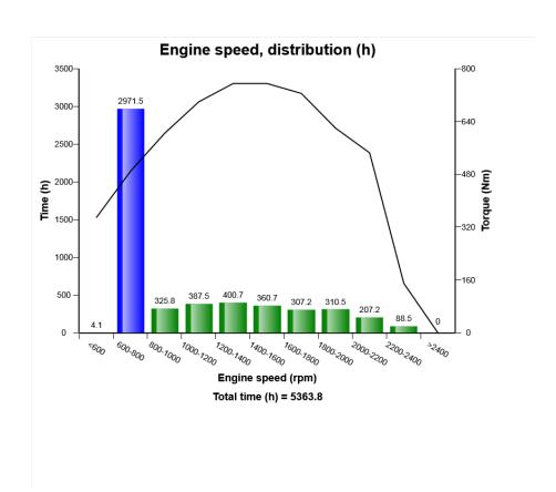
The graph describes the engine speed distribution, compared with the engine torque curve.
