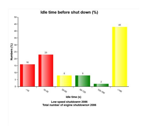
This graph shows the distribution of delayed time at low idle speed until the engine is turned off.
