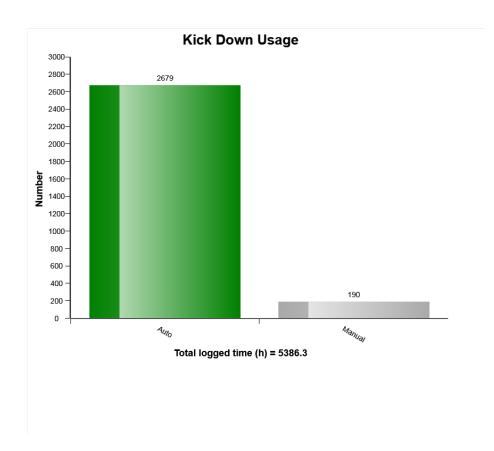
The diagram shows the distribution between Auto and Manual activations of the Kick down function.
