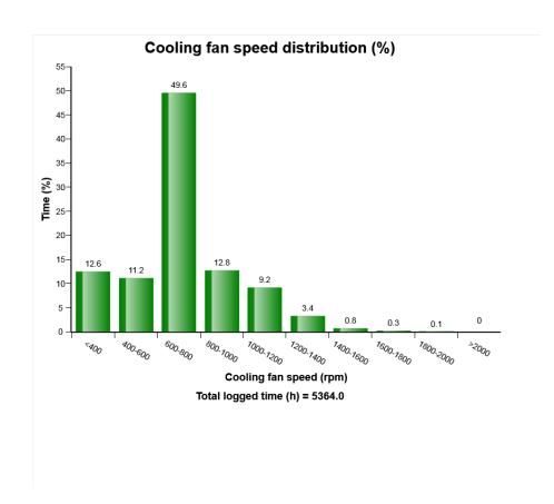
The diagram shows the time distribution for the cooling fan in different rpm ranges.
