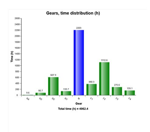
The graph describes the distribution of the usage of the different gears, expressed as total running time for each gear..
