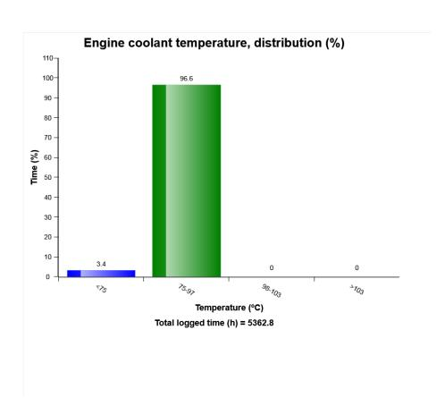
The graph shows the time distribution of the temperature, while engine running.
