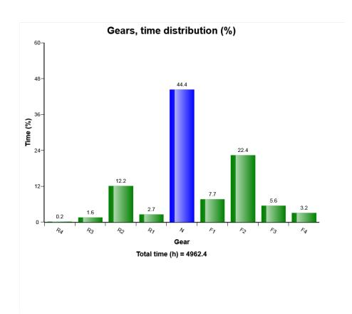
The graph describes the distribution of the usage of the different gears, expressed as percentage of total engine running time.
