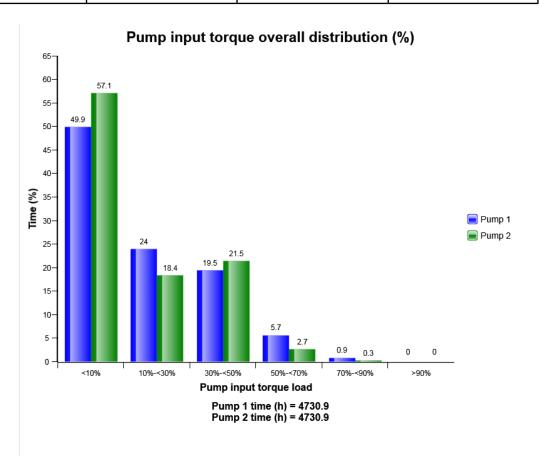
The diagram describes Pump torque load of 2 Pumps distribution.
