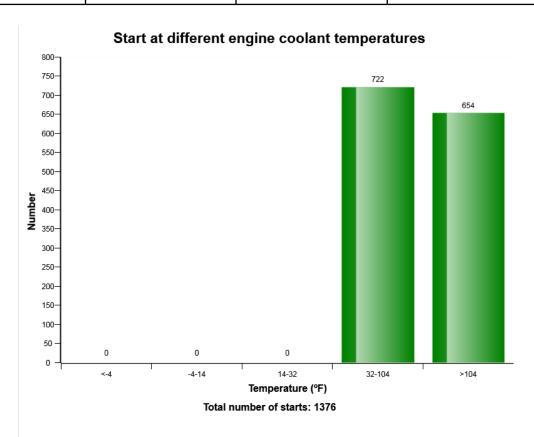
The graph shows the distribution of engine coolant temperature, at the starting moment.
