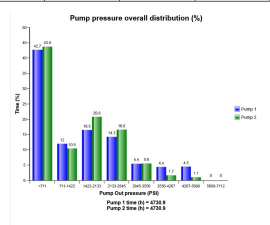
The diagram describes Pump outlet pressure of 2 Pumps distribution.
