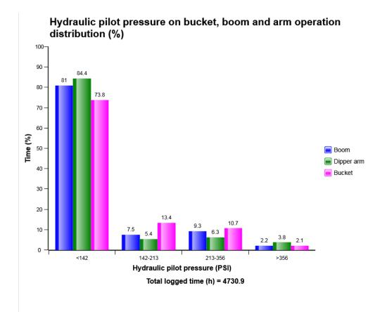
The diagram describes the distribution of hydraulic pilot pressure in specified operation
