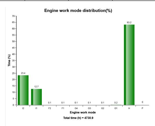
This diagram shows the distribution of the engine work mode in time percent.
