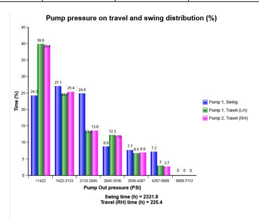
The diagram describes Pump outlet pressure of 2 Pumps for travel and swing operation distribution.
