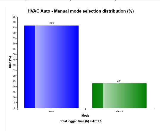
The diagram describes auto-manual mode sele ction distribution of HVAC system in machine while it Works. The share of each mode compared to Total time of HVAC operation is displayed.
