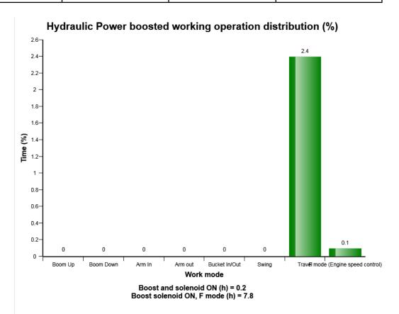
The diagram describes Power boosted operating time distribution, when main relief pressure increases on working operation modes. In this diagram, the sum of time (%) of each working operation mode can exceed 100%. It means that customer has been operated several working operations at the same time.
