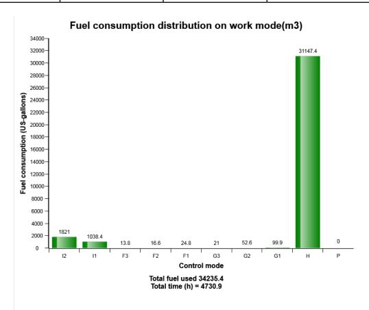
The diagram describes the amount of fuel consumed per engine speed mode distribution.
