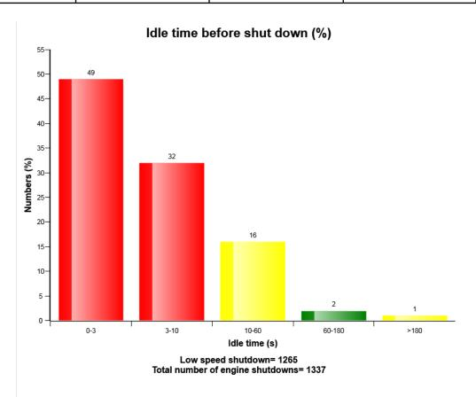
This graph shows the distribution of delayed time at low idle speed until the engine is turned off.
