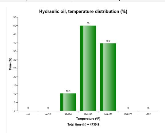
The graph shows the time distribution of the temperature, while engine running.
