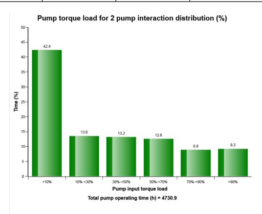
This is to see total torque load distribution of 2 pumps when it operates 2 pumps at the same time.
