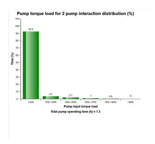
This is to see total torque load distribution of 2 pumps when it operates 2 pumps at the same time.
