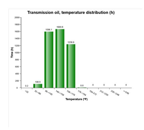
The diagram shows the transmission oil temperature in various temperature ranges. The time is displayed in the following ten temperature ranges:
