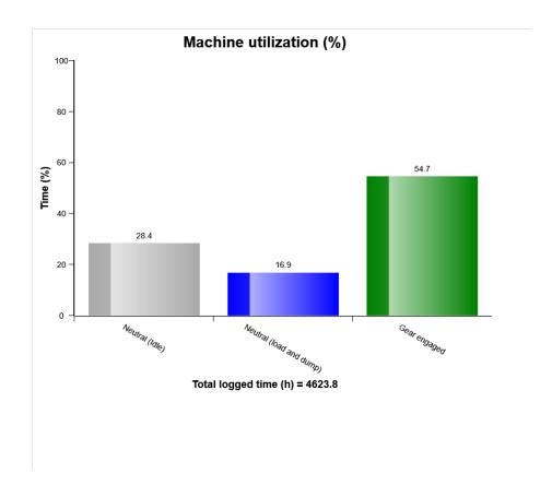
The diagram shows a simplified presentation of the machines utilization based on the relation between time in gear and time in neutral. The "Gear engaged" includes both forward and reverse gears.
