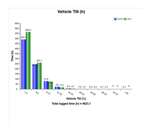
The diagram shows the distribution of the longitudinal tilt in percent (not degrees), the criteria to get registrations is that the vehicle speed exceeds 1km/h (0,62mph) and that the engine is on.
