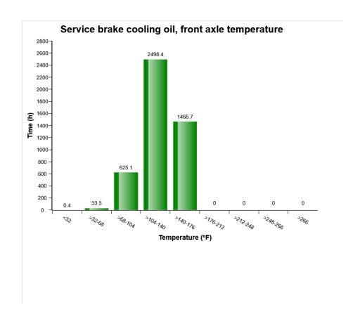
The diagram shows the front axle brake cooling oil temperature. The temperatures are divided into ranges, yellow bar (>248-266°F) and red bar (>266°F) shows abnormal temperatures. The temperature is registered in the line from the front axle to the oil cooler, that is, the warmest oil in the circuit.
