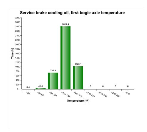
The diagram shows the first bogie axle brake cooling oil temperature. The temperatures are divided into ranges, yellow bar (>248-266°F) and red bar (>266°F) shows abnormal temperatures. The temperature is registered in the line from the first bogie axle to the oil cooler, that is, the warmest oil in the circuit.
