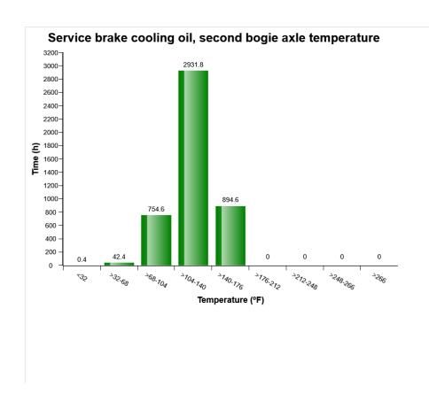
The diagram shows the front axle brake cooling oil temperature. The temperatures are divided into ranges, yellow bar (>248-266°F) and red bar (>266°F) shows abnormal temperatures. The temperature is registered in the line from the second bogie axle to the oil cooler, that is, the warmest oil in the circuit.
