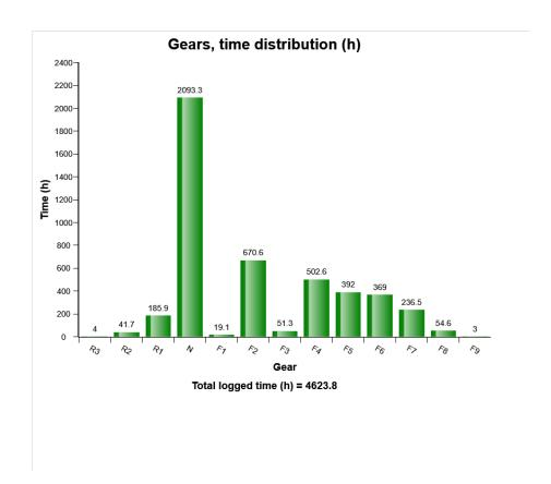
The diagram shows the time for each gear. Each bar represents a gear.
