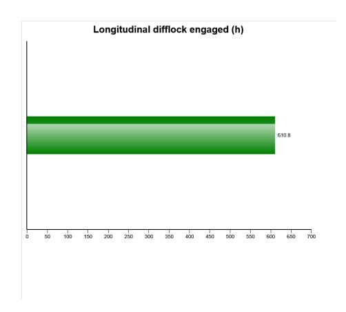
The diagram shows how long time in hours the longitudinal difflock has been engaged. The presentation only shows time when the machine is moving as this is when the wear on the difflock occurs. The difflock should always be disengage when not needed to avoid unnecessary wear.
