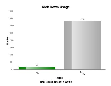
The diagram shows the distribution between Auto and Manual activations of the Kick down function.
