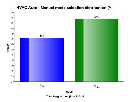
The diagram describes auto-manual mode sele ction distribution of HVAC system in machine while it Works. The share of each mode compared to Total time of HVAC operation is displayed.
