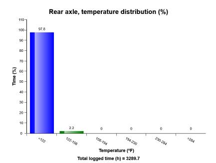
The graph shows the time distribution of the temperature, while engine running.
