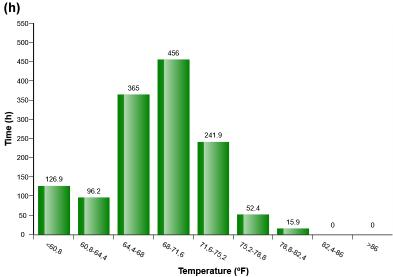
The diagram describes air temperature setting distribution for HVAC auto control mode established by operator in Cabin
