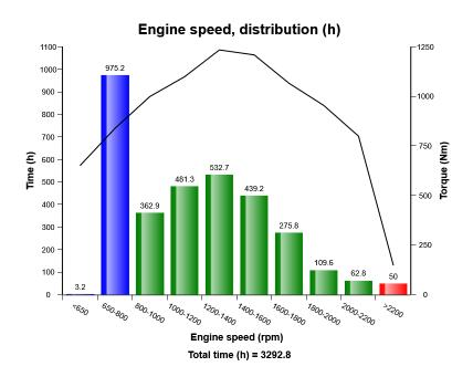
The graph describes the engine speed distribution, compared with the engine torque curve.
