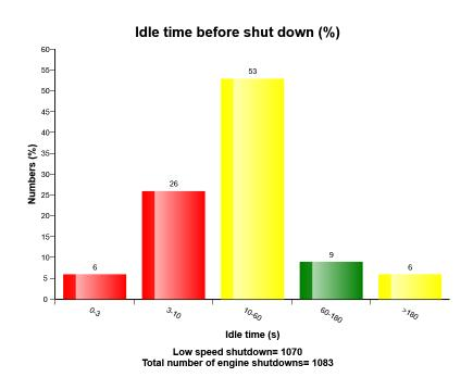
This graph shows the distribution of delayed time at low idle speed until the engine is turned off.
