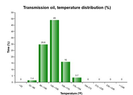
The diagram shows the transmission oil temperature in various temperature ranges. The time is displayed in the following ten temperature ranges:
