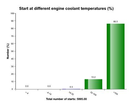
The graph shows the distribution of engine coolant temperature, at the starting moment.
