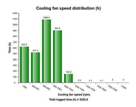
The diagram shows the time distribution for the cooling fan in different rpm ranges.
