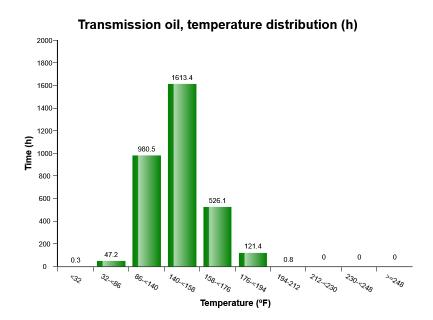
The diagram shows the transmission oil temperature in various temperature ranges. The time is displayed in the following ten temperature ranges:
