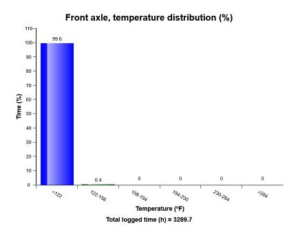
The graph shows the time distribution of the temperature, while engine running.
