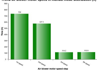
The diagram describes air blower motor speed distribution for HVAC manual control mode established by operator in Cabin.
