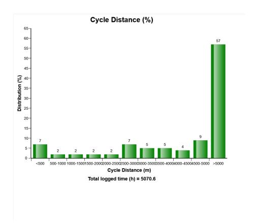
The diagram shows the distribution of the working cycle distance. The distance driven between 2 valid cycle registrations.
