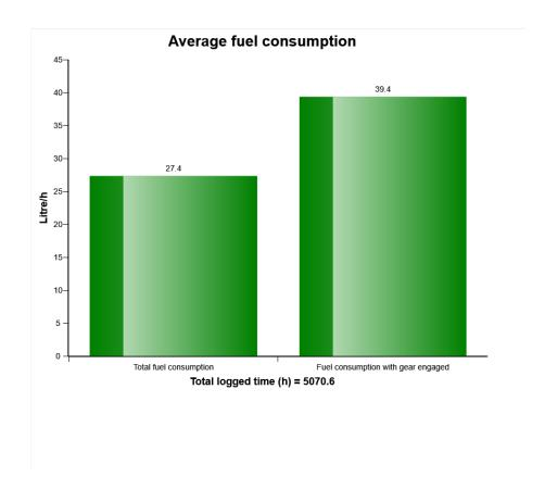
The diagram shows the total average fuel consumption versus average fuel consumption with gear engaged.
