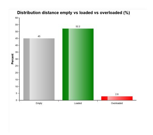
Much time operated with overload puts unnessesery stress to the machine which could lead to shorter machine life and higher repair and maintenance cost.
