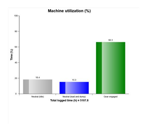
The diagram shows a simplified presentation of the machines utilization based on the relation between time in gear and time in neutral. The "Gear engaged" includes both forward and reverse gears.
