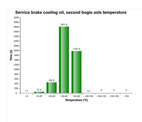
The diagram shows the Service brake cooling oil, second bogie axle temperature. The temperatures are divided into ranges, yellow bar (>120-130°C) and red bar (>130°C) shows abnormal temperatures. The temperature is registered in the line from the second bogie axle to the oil cooler, that is, the warmest oil in the circuit.
