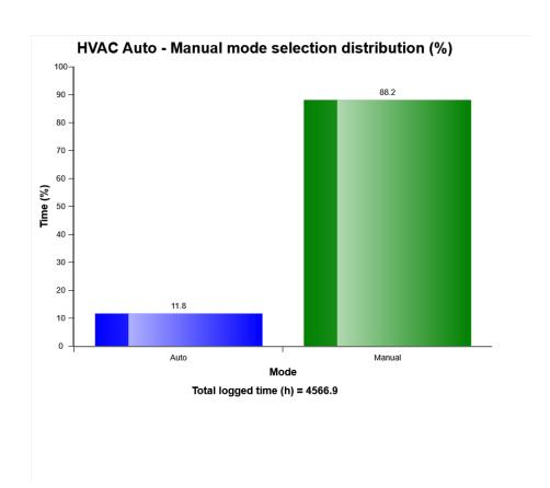
The diagram describes auto-manual mode sele ction distribution of HVAC system in machine while it Works. The share of each mode compared to Total time of HVAC operation is displayed.
