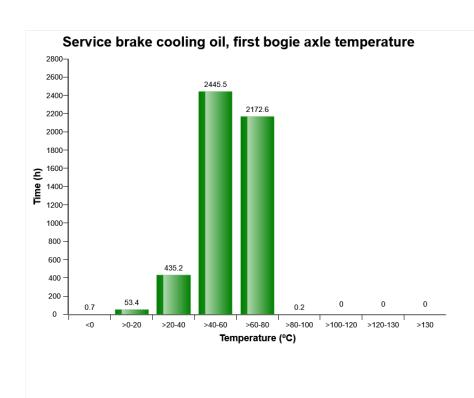
The diagram shows the first bogie axle brake cooling oil temperature. The temperatures are divided into ranges, yellow bar (>120-130°C) and red bar (>130°C) shows abnormal temperatures. The temperature is registered in the line from the first bogie axle to the oil cooler, that is, the warmest oil in the circuit.
