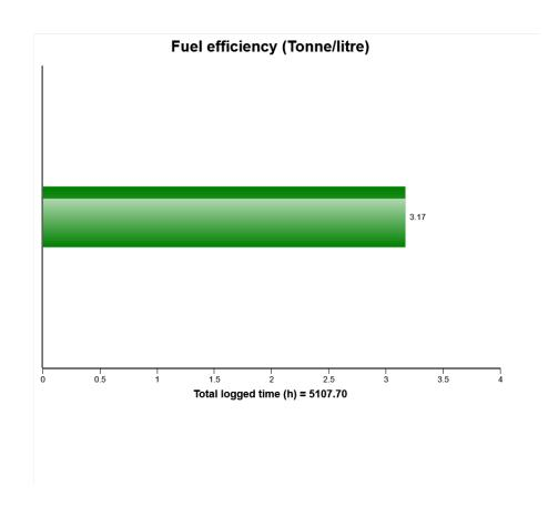
The presentation display the average produced tonne per fuel unit over the machines lifetime
