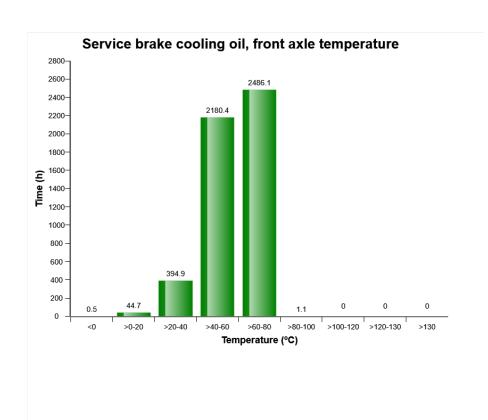
The diagram shows the front axle brake cooling oil temperature. The temperatures are divided into ranges, yellow bar (>120-130°C) and red bar (>130°C) shows abnormal temperatures. The temperature is registered in the line from the front axle to the oil cooler, that is, the warmest oil in the circuit.
